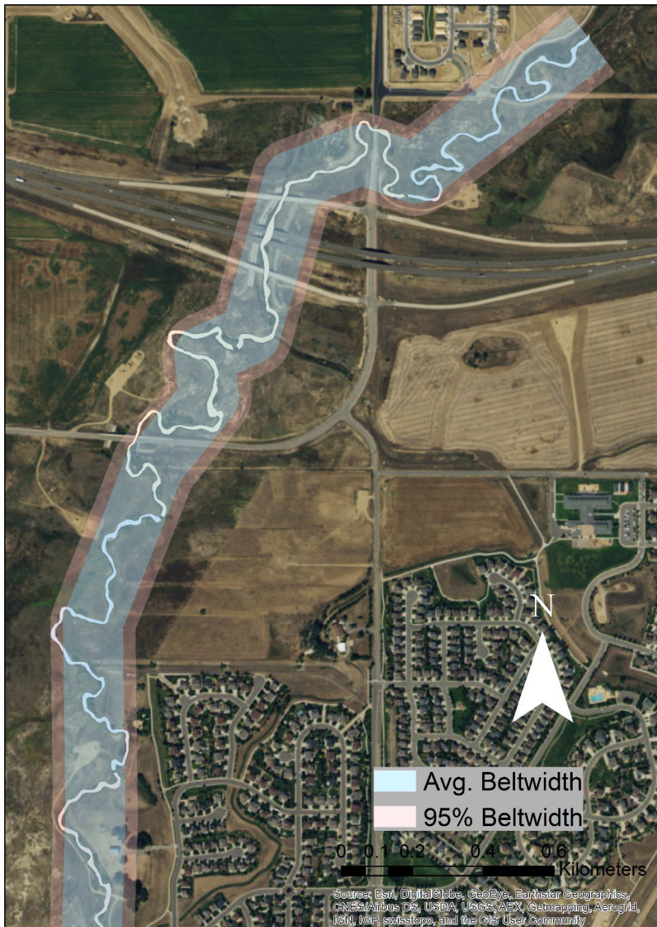
Figure 2. Estimated Average and 95 th Percentile Meander Beltwidth for Big Dry Creek through Project Area (Northern Project Area)
